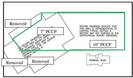
Figure 8 PCCP Thickness
